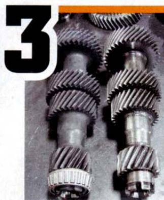
3 Our gearset was treated to a Super Finish polishing process. Compared to a stock gearset (left) it greatly reduces stress risers that can riddle the teeth and cause premature wear. In addition, it helps with lubrication and promotes quieter operation. This service sells for anywhere from $250 to $450, depending on the version of T56 that you have (Corvette or otherwise).
