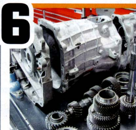
6 Here is an exploded view of our T56 before reassembly. As you can see, T56s rely on a bolt-on frontplate for easier serviceability and a rear tailhousing that houses the two overdrive gears (Fifth and Sixth) and of course, Reverse gear. Note that there are two shifter locations possible at the top of the T56. Camaros use the rear opening while Corvettes use the forward one and use a very short tailhousing.
