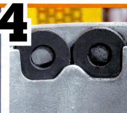
4 Using two circular magnets, a T56 is well protected against aquatic-borne materials that could wreak havoc on gears and synchronizers. T56s are one of the few transmissions in the world that boast such designs from the factory. We wiped everything down before assembly and chased every remaining particle down with a hand-held magnetic tool.
