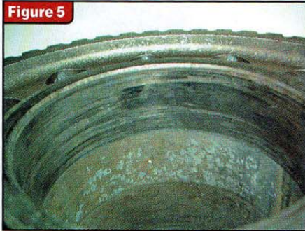
Figure 5 Internal sprocket damage
