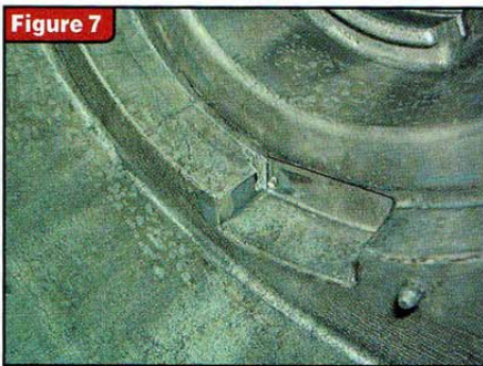
Figure 7 Hole in case caused by pump wear
