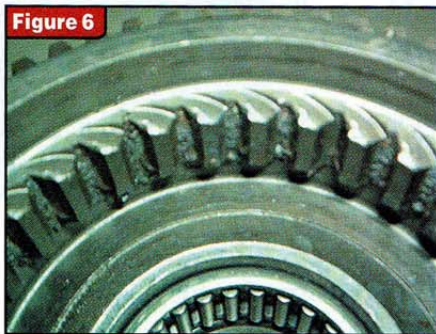
Figure 6 Internal contamination of input shaft
