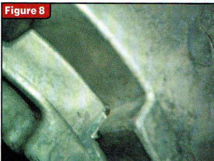
Figure 8 Oil-pump wear on the opposite side of the case caused by wear on the pump housing
