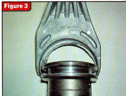
Damage to the low-range fork and hub
