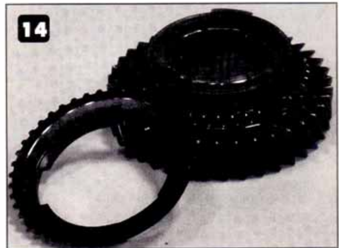
14 The double-lined synchro ring now is assembled on top of the inner single-lined cone with the locating tabs in the slots of the speed gear. 10
