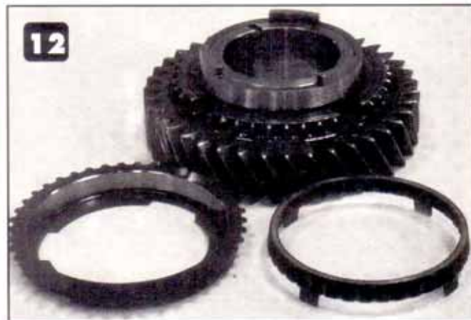
12 The single-lined inner cone is placed on the cone of the 1st-speed gear.
