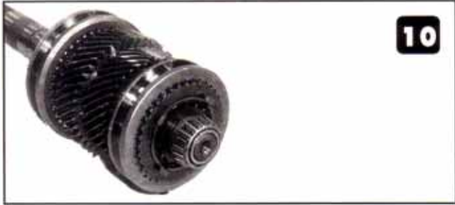
10 Here you can see the 4th-gear synchronizer components assembled on the main shaft. The arrow points to the locating tabs for the double-lined ring that index in the slots on the input or main drive gear. When assembling the input shaft to the main shaft, take care to locate the tabs properly. It doesn't take much to bend these tabs if they are not assembled properly.
