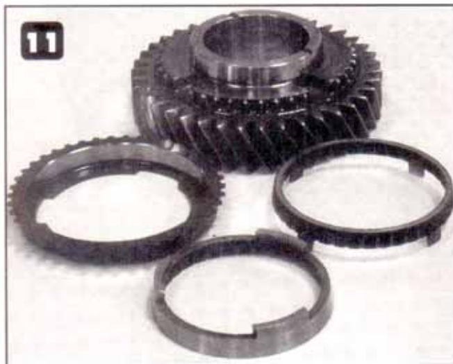
11 The 1st- and 2nd-gear synchro rings also have been modified for use in the Corvette. You can see that a cone has been added to the speed gear. There is now a single-lined inner cone in the foreground, a double-lined synchro ring on the right and a steel outer cone to the left. This gives 1st- and 2nd-speed gears triple-lined synchro assemblies.
