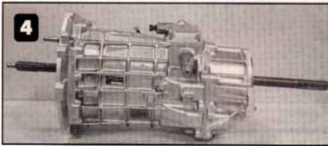
4 In this driver's-side view of the unit, the skip-shift solenoid is under the shift tower. The fill plug is in the middle of the case, and clearly visible below it is the fluid-fill label, which specifies DEXRON III synthetic ATF. This unit uses carbon-fiber rings and must be filled with synthetic ATF only . The use of any other fluid will cause premature failure and shift problems.
