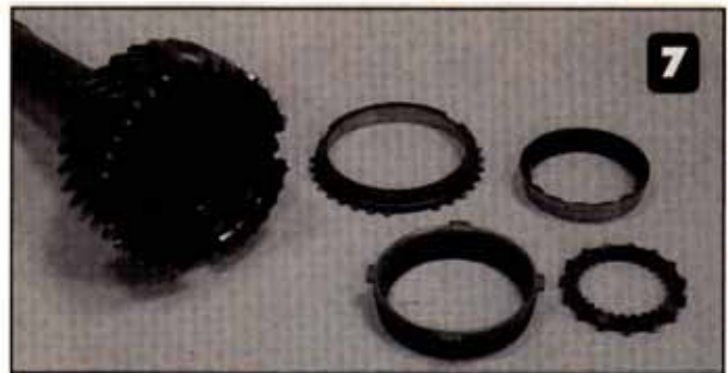
7 This view shows the inner and outer synchro cones, the double-lined 4th-gear synchro ring with four locating tabs, and the splined inner washer. On the F-body T-56, 3rd- and 4th-gear synchro rings have only a single lining.
